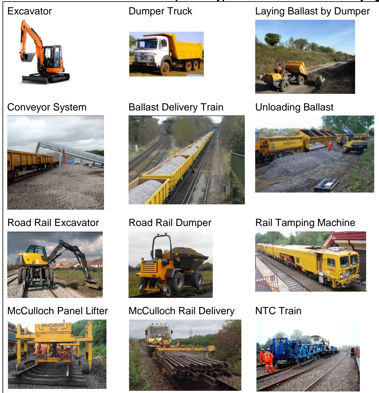
Plate 4.1 Examples of Typical Plant Used for Track Laying
